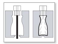
Figure 2: In extrusion blow molding, a molten tube of plastic is extruded into a mold cavity and inflated with compressed air
