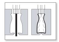
Figure 5: Continuous extrusion blow molding. The parison is extruded through a die (left), and the mold closes on the tube of plastic. The parison is then inflated (right) to force the plastic to the contours of the tool.
