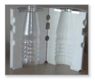
Figure 11: To mold the PET bottle, this hybrid insert uses a cylindrical design.
