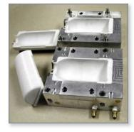
Figure 9: FDM hybrid tool with contoured inserts.
