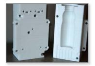
Figure 3: Polycarbonate blow mold made from the FDM process.
