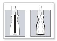
Figure 6: Intermittent extrusion blow molding. The parison is extruded within the mold cavity (left) and inflated with air pressure (right).
