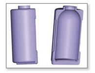
Figure 10: CAD data for a contoured insert that is mounted in a machined mold base
