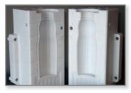
Figure 8: FDM blow molding tool made from polycarbonate.
