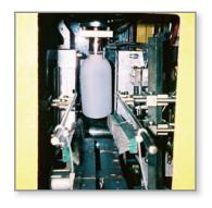
Figure 14: Prototype hybrid FDM tool opens and HDPE bottle is ejected.
