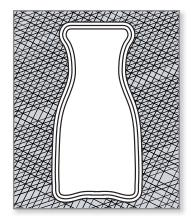
Figure 12: Increasing the number of contour passes reduces porosity and improves part quality.
